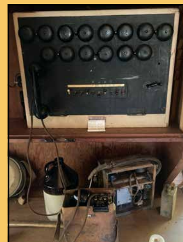
This switchboard was the hub of fire information from the manned fire lookouts on nearby buttes. Bikepacking the Oregon Timber Trail. Photo by Tom Diegel
