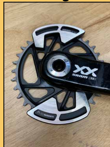
SRAM Transmission has chainring mounted bashguards. Photo by Tom Jow
