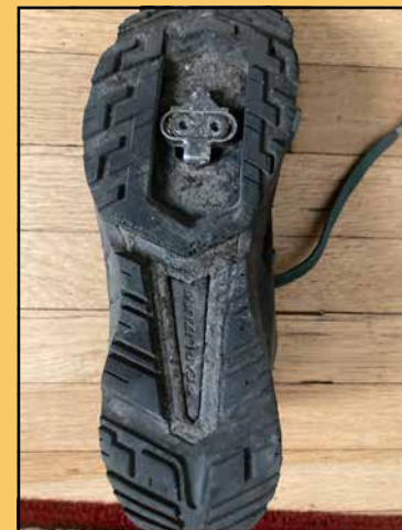
The Canyon's spd cleat is slightly more recessed so the rubber sole contacts before the metal cleat. Photo by Tom Diegel
