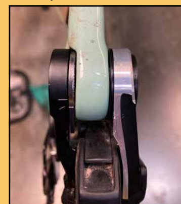
The SRAM Transmission derailleur mount sandwiches the frame dropout for strength. Photo by Tom Jow
