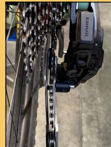
With SRAM Transmission, the derailleur cage is designed for better alignment with the chainring. Photo by Tom Jow
