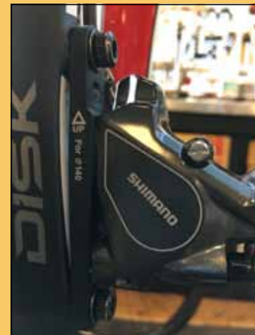
The Shimano Flat Mount Disc Brake System requires a new mounting system on the frame and results in a lower profile fork. Photo by Tom Jow
