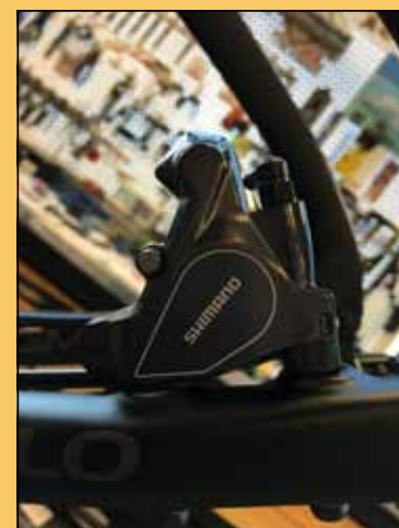
The Shimano flat mount rear disc brake. Photo by Tom Jow
