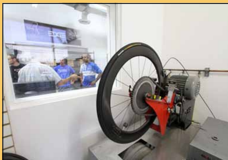
Left: The ENVE 45's are a solid choice for road or cross. Above: ENVE's new machine for testing heat dissipation. Photos: courtesy ENVE Composites.
