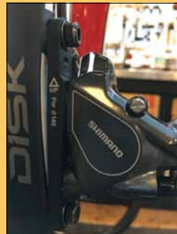
The Shimano Flat Mount Disc Brake System requires a new mounting system on the frame and results in a lower profile fork. Photo by Tom Jow
