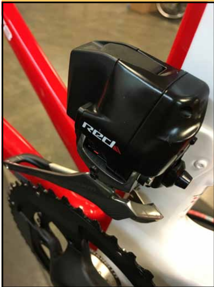
SRAM eTap wireless electronic front derailleur. Photo by Tom Jow
