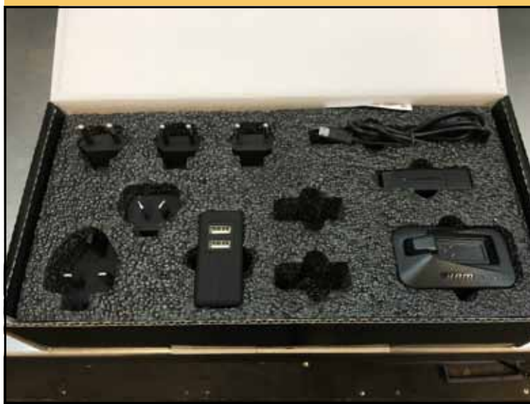
SRAM eTap wireless electronic shifting system charging system. Photo by Tom Jow
