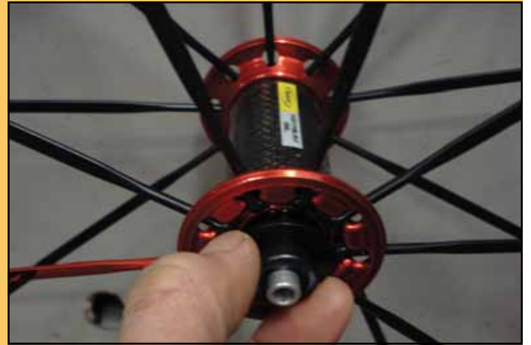
Wheels: Rotate wheel axles to test for bearing wear.
