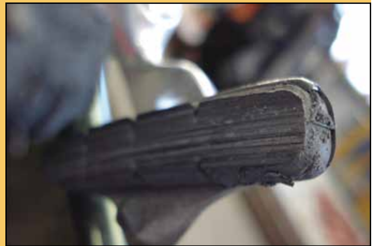
Brakes: Brake pads worn beyond wear grooves.
