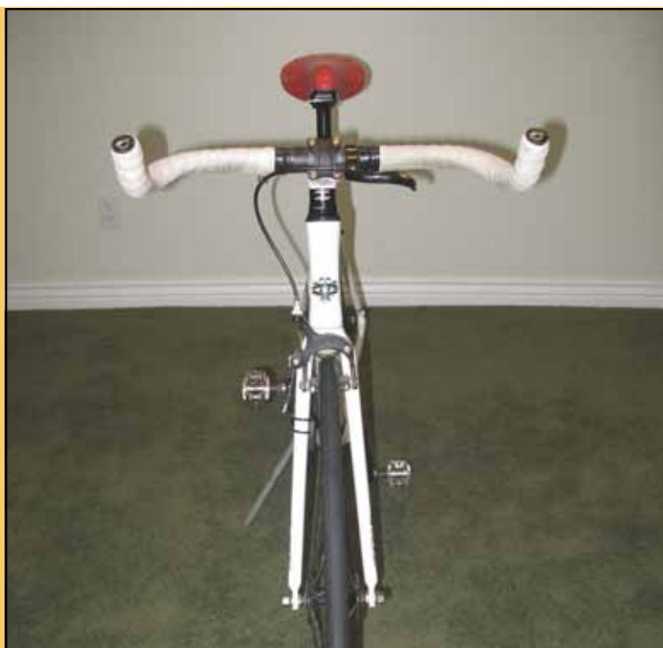
The epitome of simplicity. No derailleurs, just a frame, crank, pedals, wheels, handlebar, seat, and one brake.
